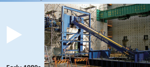
Early 1980s Original research and development of BRBs by Nippon Steel Corporation 1987
