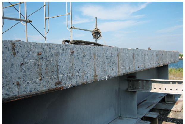
図19 供試体切断状況 Fig. 19 Cutting plane of the specimen
