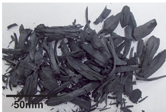
図6 乾留後バイオマスチップ外観 Fig. 6 Image of biomass chip after distillation
