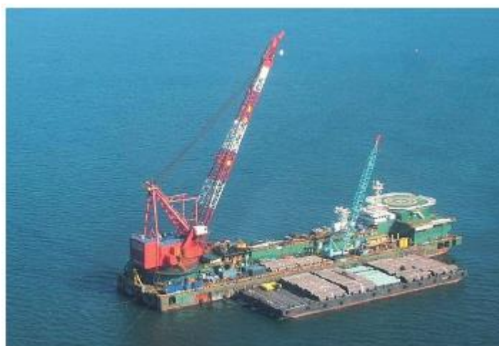
Fig. 1: Specialized pipeline-laying barge “Kuroshio No. 2” owned by NSENGI (photo)
