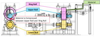
Figure 4 Component of Nippon Steel & Sumikin Engineering Squeezer
