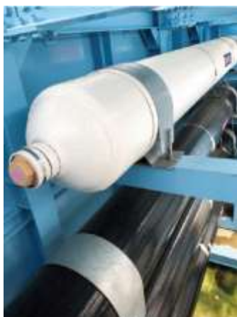
Figure 3 Composite storage vessels White: Type 2 Black: Type 3
