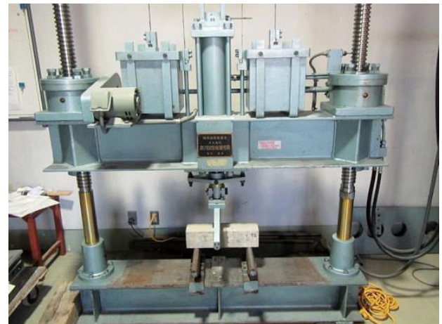
Fig. 8 Machinery for Three-Point Bending Flexural Test
