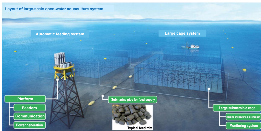
Figure 2 Layout of large-scale open-water aquaculture system
