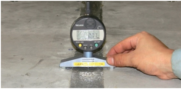
図6 沈下量測定状況 Fig. 6 Appearance of Measuring Settlement
