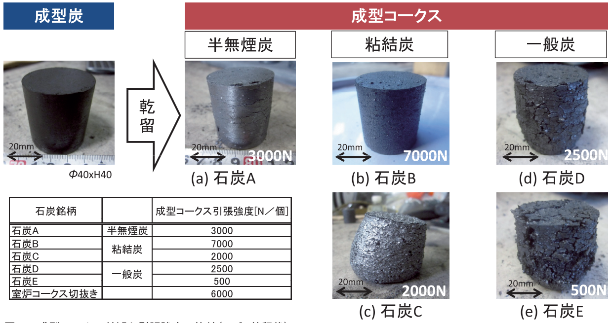
図7 成型コークス外観と引張強度の比較(900℃乾留後) Fig. 7 Comparison of appearance and tensile strength of formed coke (after carbonization at 900°C)
