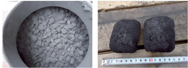
図18 溶融炉向け成型コークスの外観 Fig.18 Image of formed coke briquette for direct melting system
