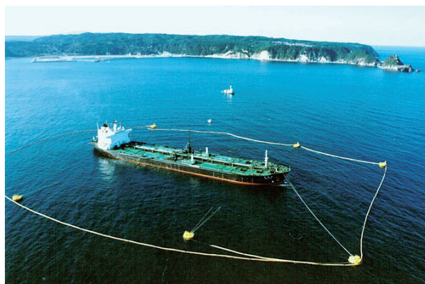
図2-1 10万DWTタンカー浮標式多点係留設備(岩手県久慈湾、日本地下石油備蓄(株)提供)(写真) Fig. 2-1 Multi-Buoy Mooring berth for 100,000 DWT class tanker in Kuji bay, Iwate pref. (Photo by Japan Underground Oil Storage Co.,Ltd.)
