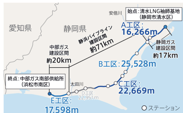
図12 静浜幹線建設工事路線図 fig.12 Route map of the Shizuoka trunk line construction
